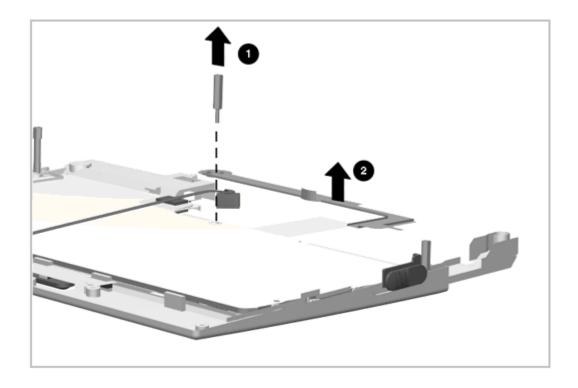
Figure 5-44. Removing the CD-ROM Eject Bar and Standoff
